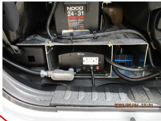
Inverter and deep cycle AGM battery to be install/mounted in front top vertical storage compartment
