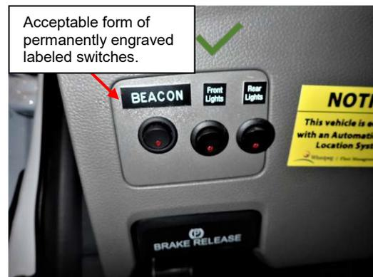
**Not Acceptable – Not Permanently Label Picture above shows example of permanent engraved label switches.**
